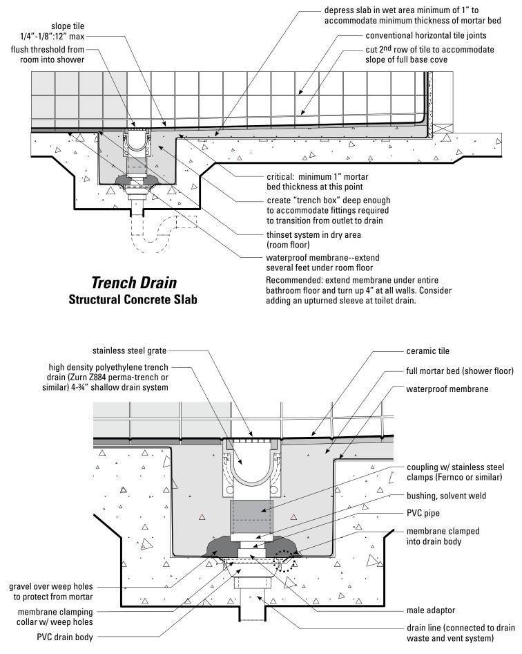
Suggested Detail: Concrete Slab
