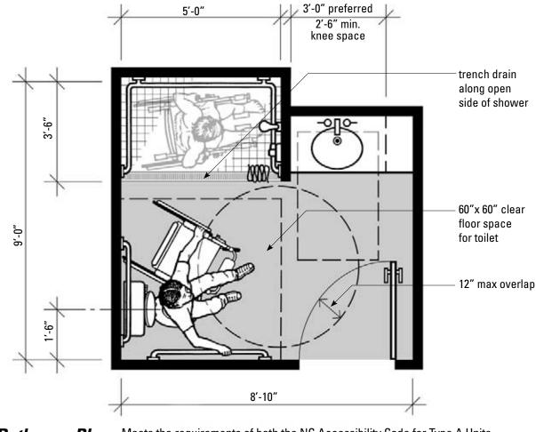
Sample Bathroom Plan with Curbless Shower and Trench Drain Meets the requirements of both the NC Accessibility Code for Type A Units and the NC Housing Finance Agency's Qualified Allocation Plan (QAP). Smaller bathroom designs are possible when full accessibility is not needed. See the QAP Bathroom Tech Sheet on the CUD website for other options.
